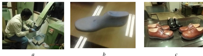
Figure 1. Last Making (a and b) and Full shoes (c)
