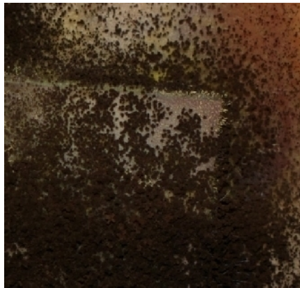
Figure 1. Aspergillus niger and Aspergillus flavus moulds spontaneously grown on the wet-white leather sample tanned with resorcinol-oxazolidine after 21 days
