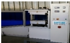
Figure 1. Electrically heated press, TP 600
