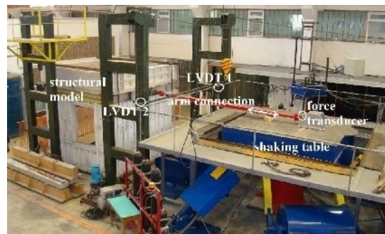
Figure 2. Structural model laterally connected to shaking table
