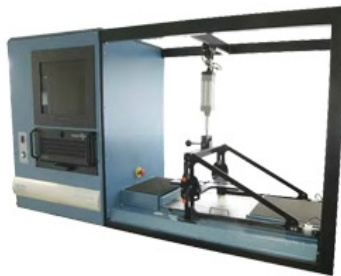
Figure 3. Slip resistance tester
