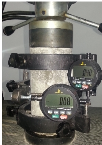
Figure 1. Measuring modulus of elasticity in compression
