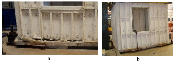
Figure 4. a) Failure of the base connection; b) additional connection of the structural model
